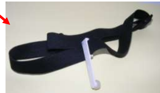
Eye lens dosimeter (prototype-developed by RADCARD in the frame ORAMED project)
