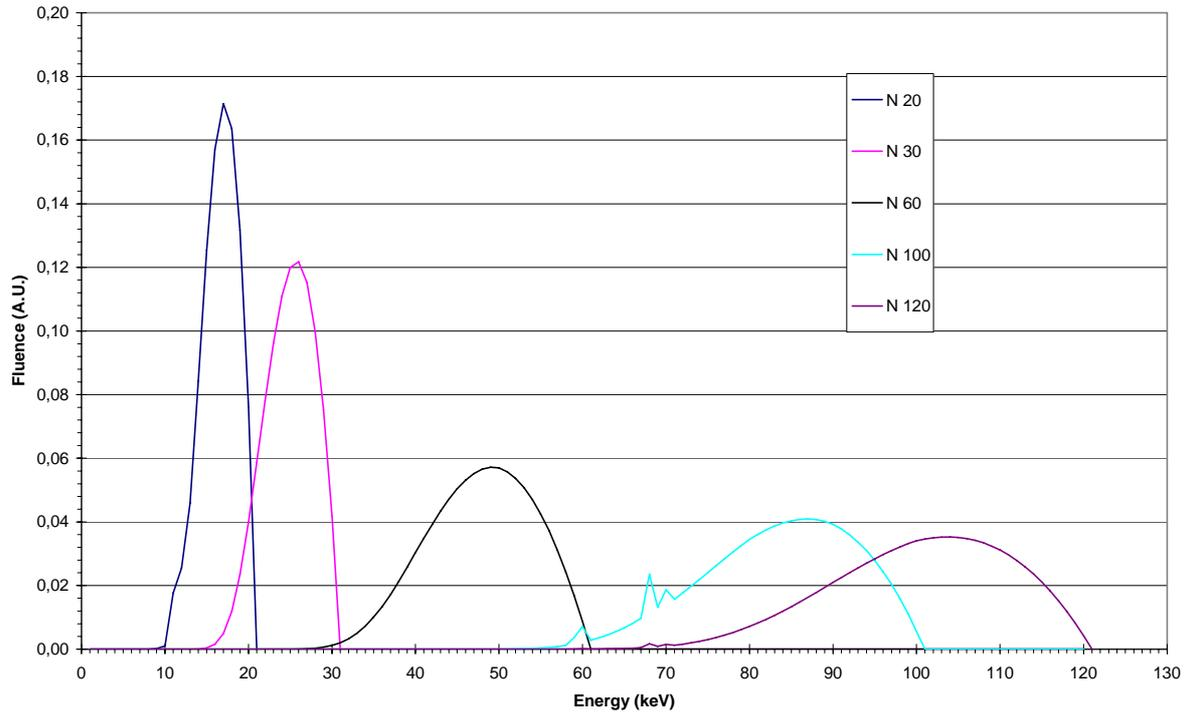
Figure A1: Spectra of narrow spectrum series described in ISO 4037
