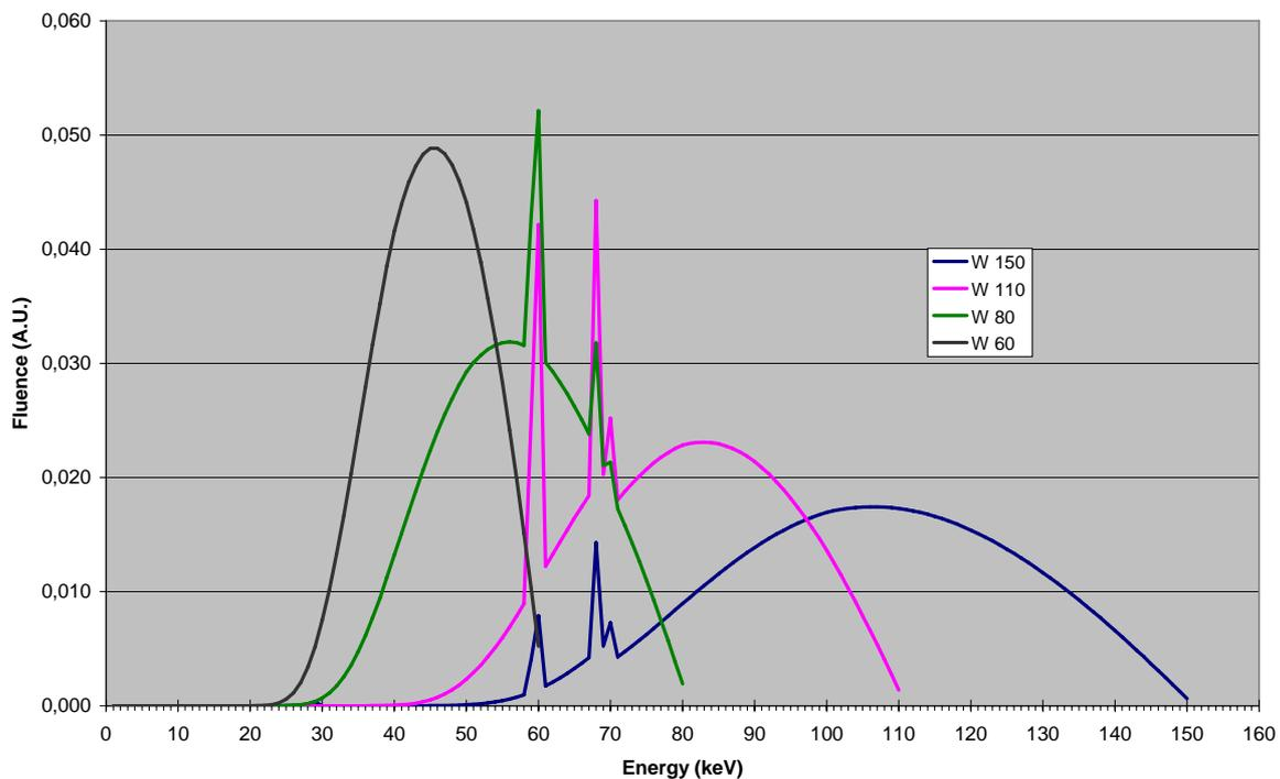
Figure 2: Spectra for a few radiation fields (wide-spectrum series of ISO 4037)
