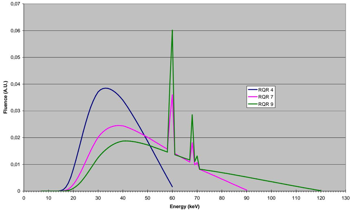
Figure 3: spectra of RQR radiation field described in IEC 61267
